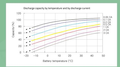
This testing graph shows us the different discharge capacity under temperature and C rate.
