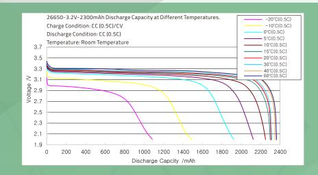
This testing graph shows us the different discharge capacity under temperature influence.
